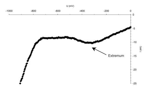
Fig. 3. Example of a current-voltage curve (soil No. 568; soil water content 46.7%) obtained with the three-electrode system. There is a relative extremum in the range of potentials of quasiplateau.
