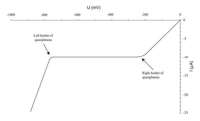
Fig. 2. Idealized current-voltage curve and definition of right and left borders of quasiplateau.
