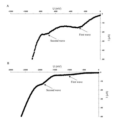
**Rys. 4.** Examples of current-voltage curves where two waves can be observed. These waves can be evidence that the reduction of molecular oxygen in not the unique electrochemical reaction in the system. A) three-electrode system in soil 565; soil water content 53.7%; B) three-electrode system in soil 606; soil water content 40.2%.
